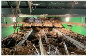
CREATE EVEN DISTRIBUTION Adjust Auger Beds First Install Concave Covers if Necessary MONITOR AND ADJUST AS CROP MOISTURE CHANGES INSTALL RAISED FRONT CHAFFER COVERS Cleans Grain Earlier
